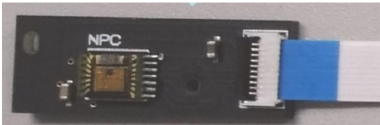
FFC Cable connecting encoder board and breakout board.
